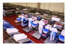
According to customer requirements, weighing stations for bulk products can be designed in a way that a final check for contaminants is performed before products are weighed into plastic-covered trays.
