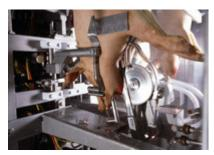
SFK's Throat opener, bung dropper and ham splitter is designed to operate at high capacities and to handle natural anatomic variations in pig dimensions.
