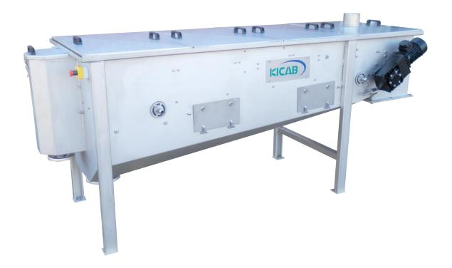
Stingray SBT mechanical thickener combines traditional proven technology with new innovation, design & manufacturing. Mechanical thickening enables big savings in transport, dewatering & digestion efficiency.
