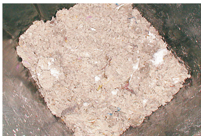
End product: washed, pressed and shredded screenings
