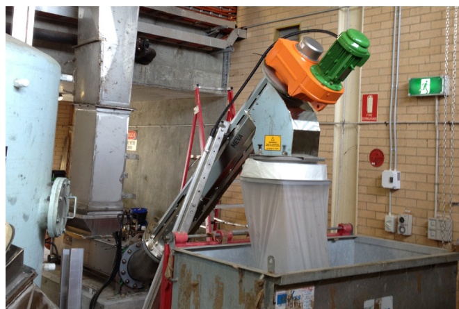
Meva CPS with Longofill equipment for improved hygiene
