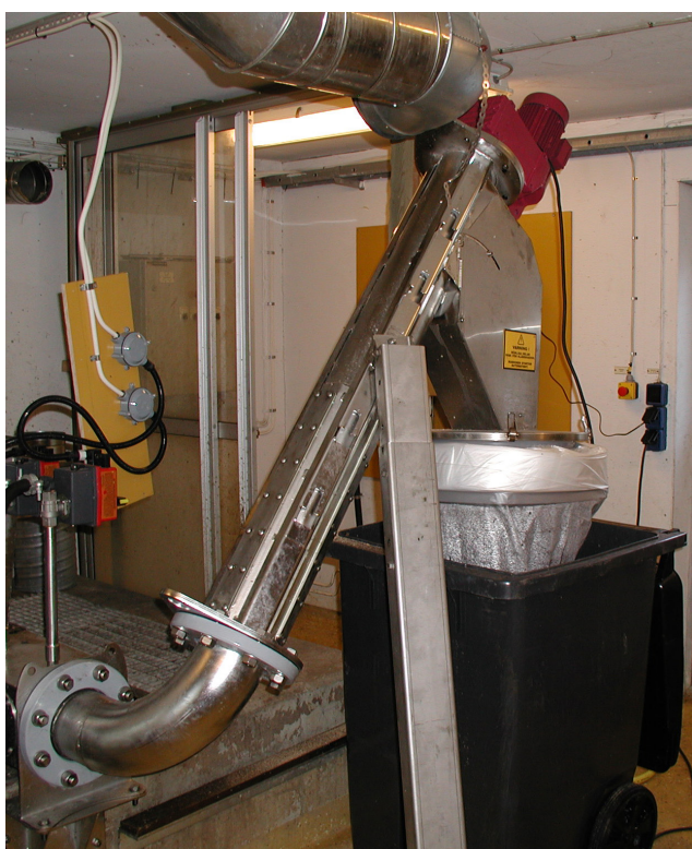
Meva Counter Pressure Screw CPS with longofill
