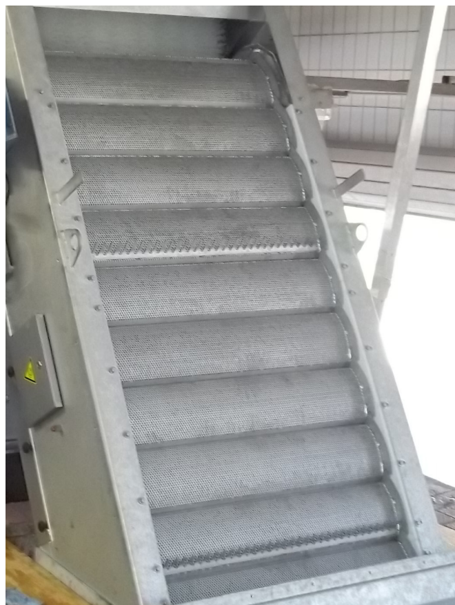
Meva MPS is delivered with a seamless belt
