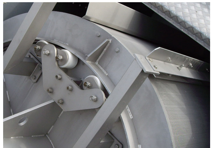
Stable roll bearings in the Meva MDS
